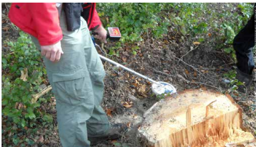
Individual small hotspots are identified with the metal searching device.
