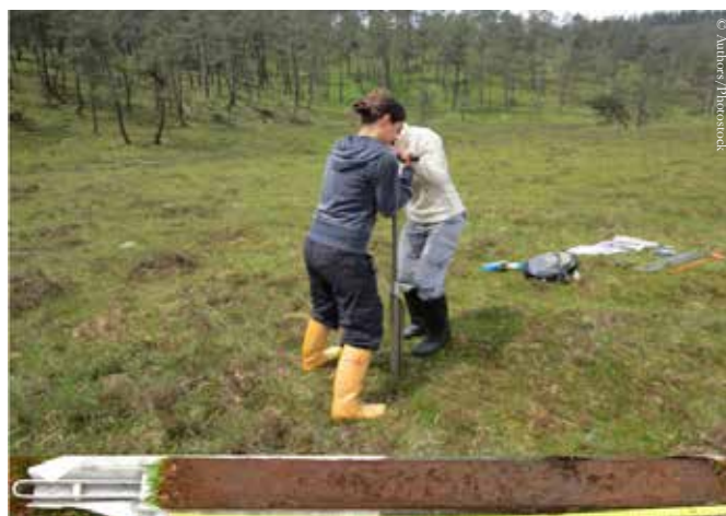
Collecting a peat core in the Tremoal do Pedrido mire (Xistral Mountains, NW Spain). An example of a core sampled with a Waardenar corer is shown at the bottom of the picture.
