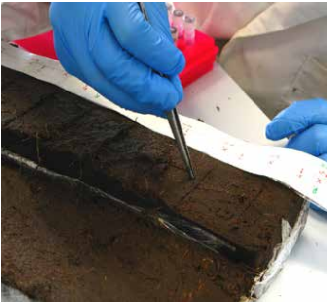
Spain, North West. Peat core sampling to investigate into the microbial composition of the peat
