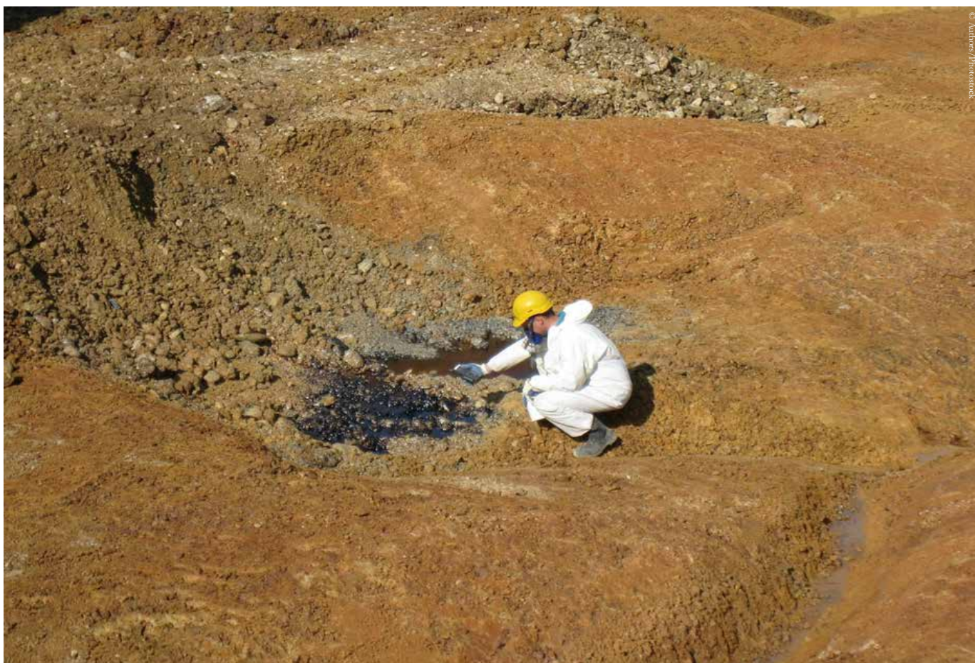
Accumulation of pollutants (black) on an impermeable marl layer (yellow-orange)
